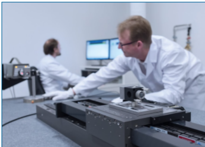
Figure 8. A technician performs metrology and calibration on a linear stage.
